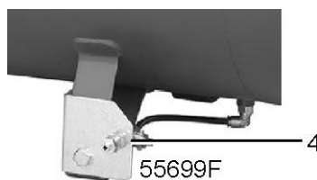
Drain valve of air receiver
