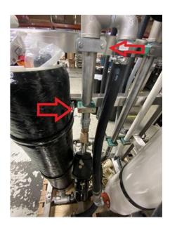
**6.** Remove Solenoid E and the pipe it is connected to.
