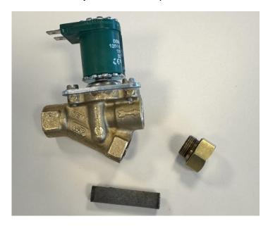
**Step 3**: Run the strainer under the faucet until clean. Make sure there is no debris in the valve itself.
