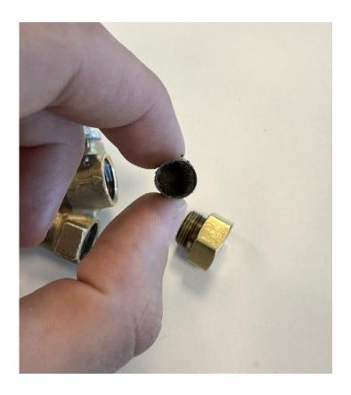
**Step 4**: Re-install the y-strainer into the valve. Make sure it is seated firmly before installing the cap.
