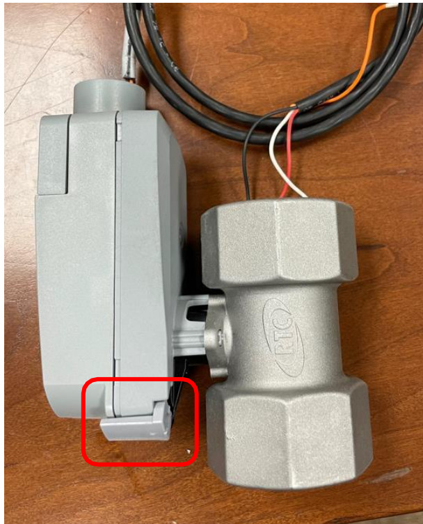
Figure 11 – Safety Stop is circled in red. Stop can be removed without any tools. Safety Stop snaps onto actuator.
