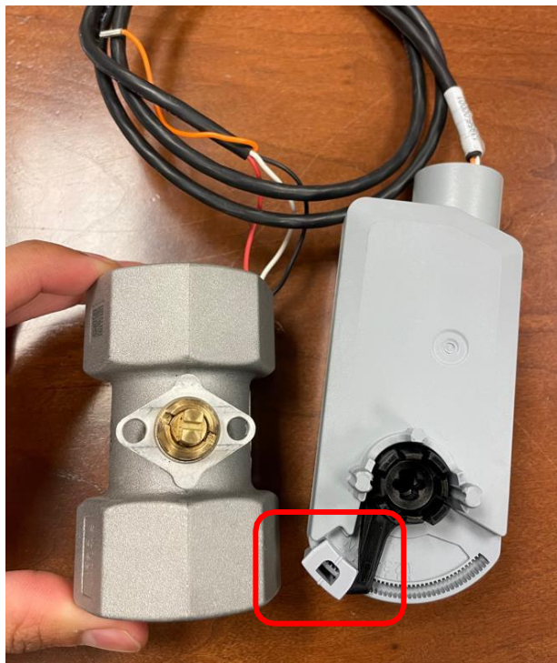
Figure 12 – to adjust the Safety Stop, during HIGH fire operation, move the stop to a new position along the arc. DO NOT remove the actuator from the valve during HIGH fire operation. The black level will rest against the stop during LOW fire operation.
