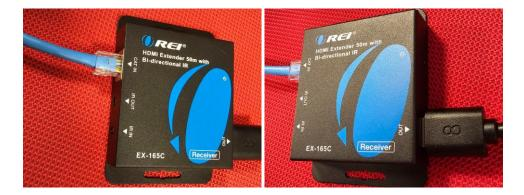
4. Replace the HDMI cable from the HDMI to Ethernet (REI) receiver to the TV with the one from the Mac Mini and monitor. This will determine if the HDMI cable was damaged and needed to be replaced.
