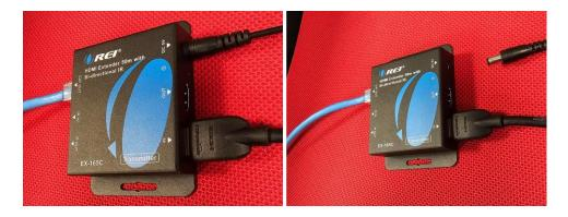
Inspect the receiver of the HDMI to Ethernet (REI) transmitter and HDMI cable connected to the TV. Pull the HDMI and transmitter apart to inspect more.
