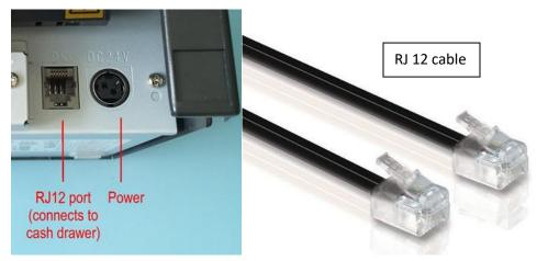
2. Connect the 3 pin DC 24v power Adaptor into the DC 24V on the Printer.
