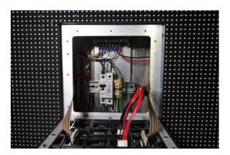
• The blue and black/green data cables in Panel A must be connected to the corresponding ports on the Receiving Card in Panel B.
