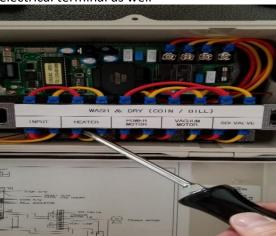
Remove the Fan line from the board.
