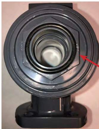
Motor Separated From PVC
