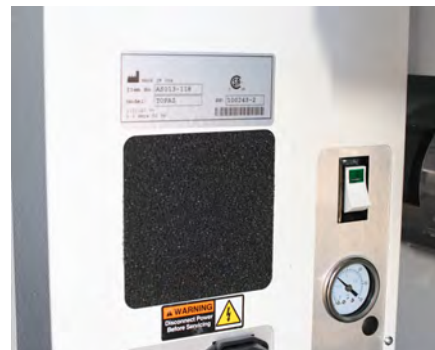
Oxygen Concentrator Air Filter with Splash Guard Removed
