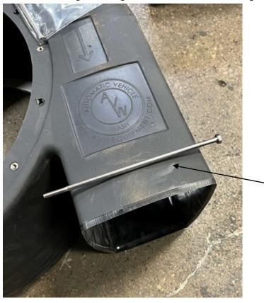
Nozzle is not pictured – make sure these bolts go through both the nozzle and housing.
