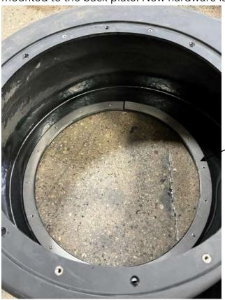
Steel ring to be mounted to the back plate of blower.
