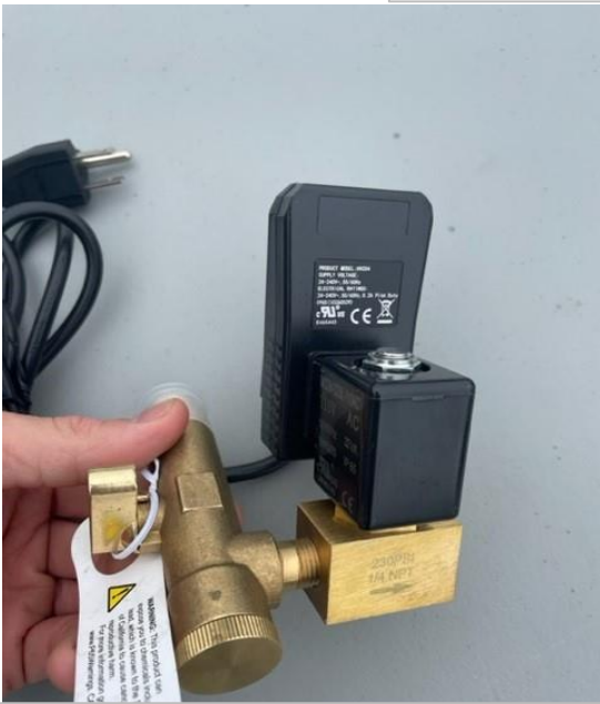
Figure 2 - MCDV25 auto drain. Note strainer plug is towards the auto drain.
