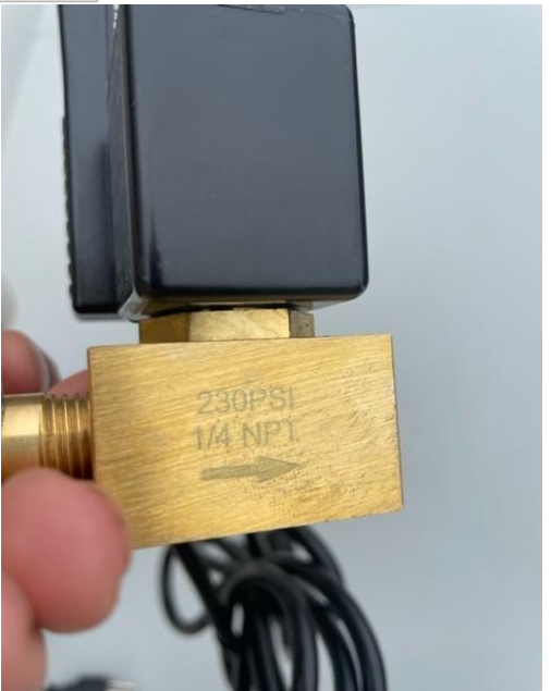
Figure 3 - note direction of flow on auto drain
