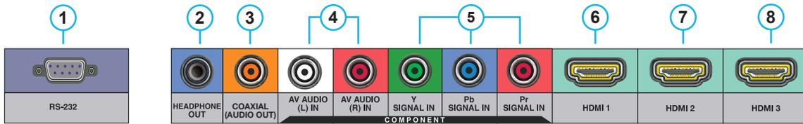
1. **RS-232C** - Long established standard connection (“C” is the current version) that describes the physical interface and protocol for relatively slow data communications between computers and related devices.
